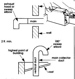
Do **Not** install screening cap over end of duct.
